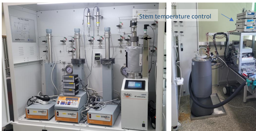
Figure 1: Measurement system for specific heat: sample preparation and injection part (left), and calorimetry part (right).
