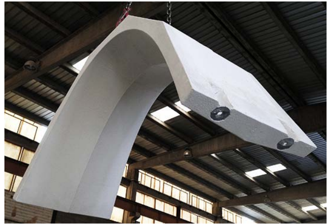
9 Final GRC panel suspended after demoulding.
