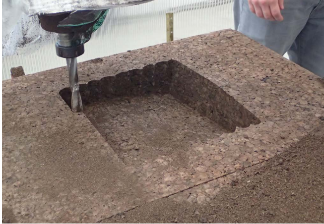
10 Robotic milling the outer surface of the cork panels.
