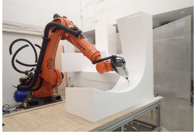
7 Robotic trimming the contours of the EPS moulds.
