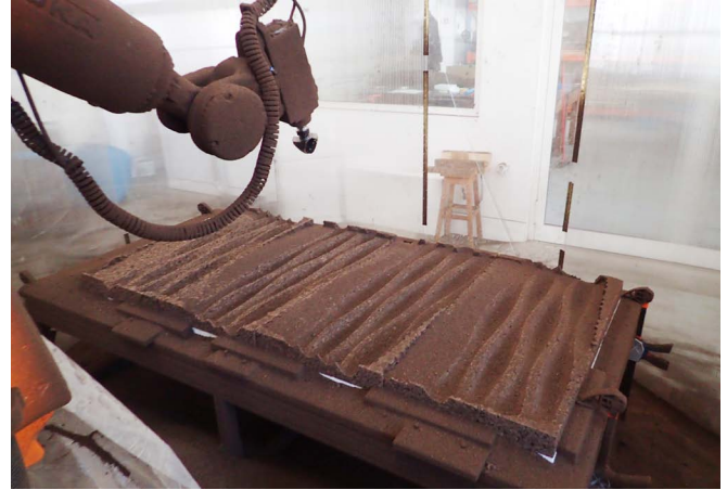
11 Robotic engraving of the texture.
