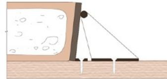
Flexible mold system for earth-based material.
