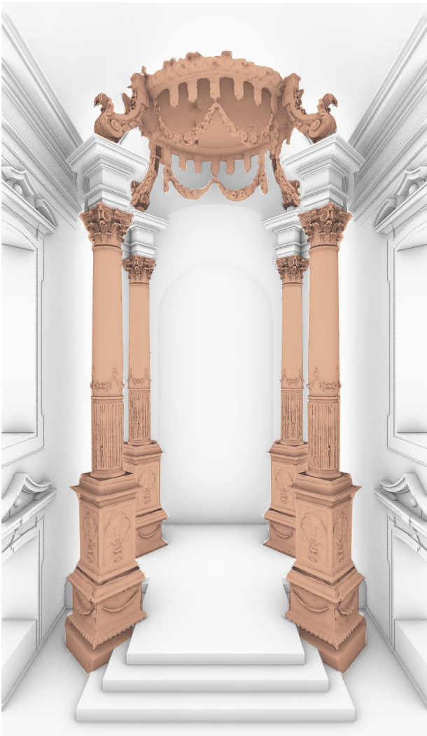
Figure 15: Reconstruction of the Baldachin: the area painted in orange refers to the photogrammetry mesh model, while the rest is explicitly modelled.
