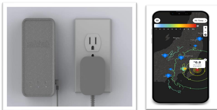
Figure 7. Safe-hub sensor for damage detection of structures based on modal parameters.
