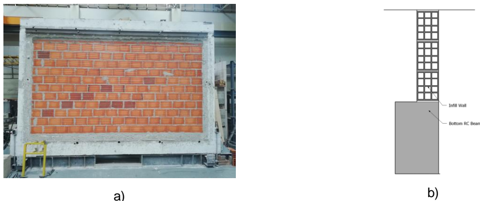
Figure 1. Infilled RC frame without retrofitting: a) general view before retrofitting; and b) profile view.
