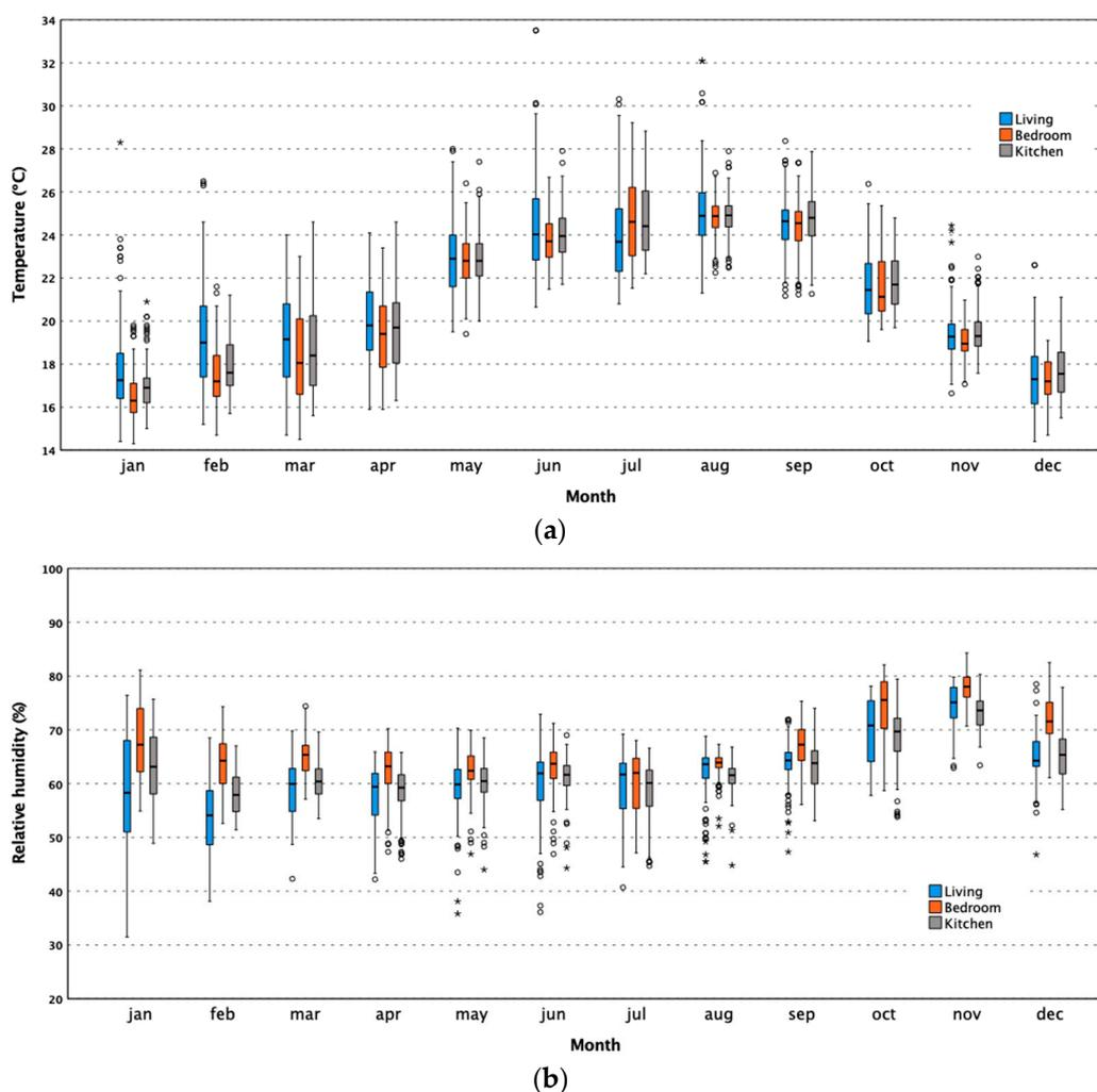
**Figure 11.** Box plot representation of monthly records inside the compartments: (a) temperature; (b) relative humidity.
