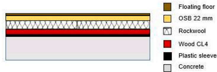
**Figure 5.** Construction solution for the floor of the house under study.
