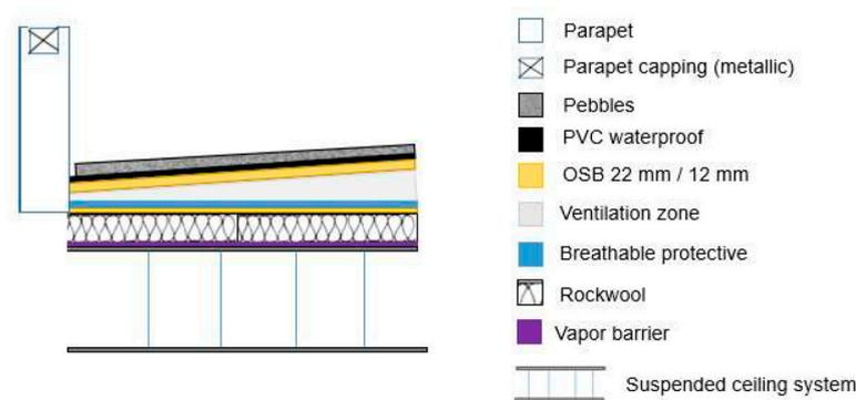
**Figure 6.** Constructive solution for the roof of the house under study.
