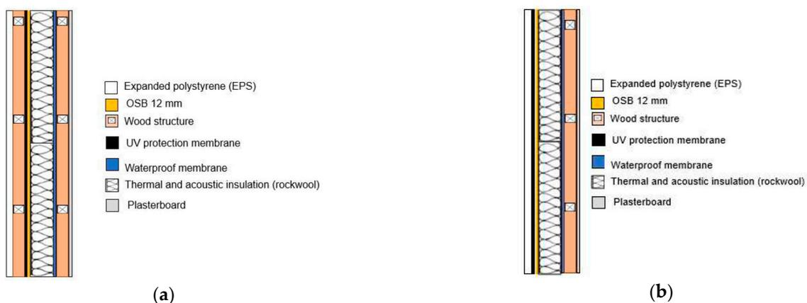
**Figure 4.** (a) Composition of the wall (system A); (b) composition of the wall (system B).
