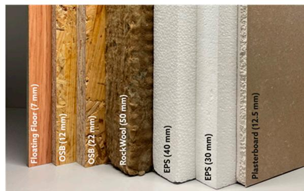
**Figure 7.** Materials used in walls and floor in the house under study.
