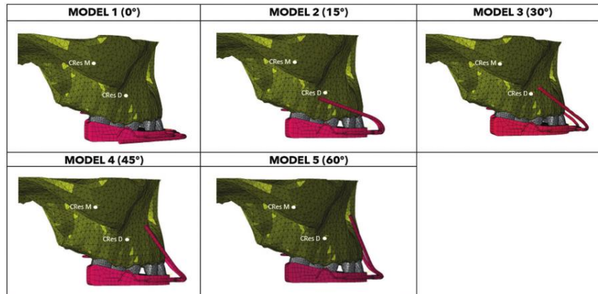
Fig. 1: Finite element model where the force lines of action used for each of the five models are indicated (M1 (0°), M2 (15°), M3 (30°), M4 (45°) and M5 (60°)).
