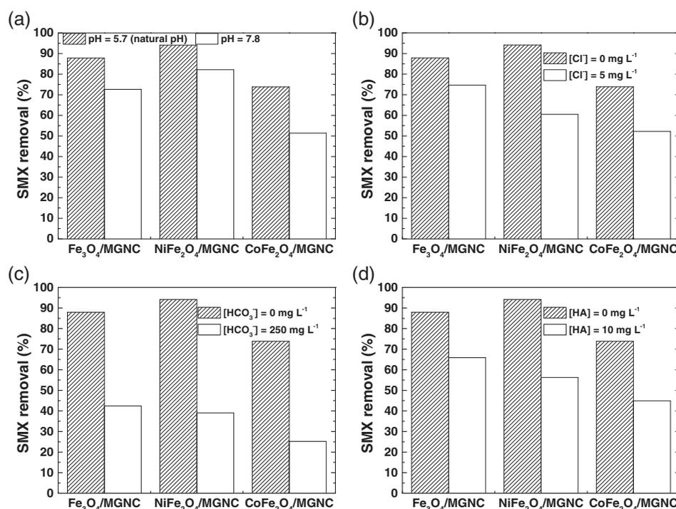
**Figure 3.** Effect of (a) pH, (b) chlorides, (c) bicarbonates, and (d) humic acid (HA), on the removal of sulfamethoxazole (SMX) obtained after 2 h in activated persulfate oxidation experiments performed in ultrapure water, with the magnetic graphitic nanocomposite (MGNC) materials. Operating conditions as given in Fig. 1.
