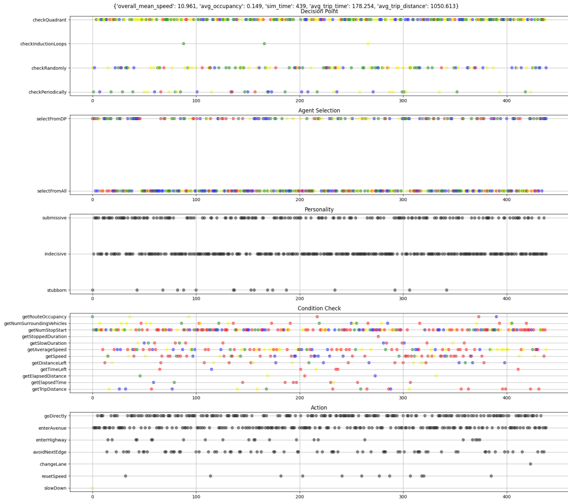
Figure 5.9: Random: Best Result Action Graph. The graph displays, for each timestep, the option chosen for each block type (Decision Point, Agent Selection, Personality, Condition Check, and Action). The coloured dots also represent the value option associated with each block option choice. It shows a somewhat contingent block option choice and scattered value option choice.
