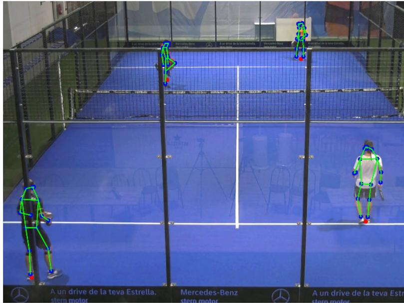
Figure 4.8: Example of pose and position estimation on a frame from the dataset gathered.
