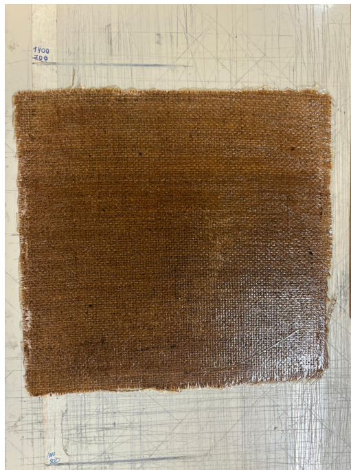
Figure 4.10: Final Jute-Reinforced PLA Composite Samples After Molding.
