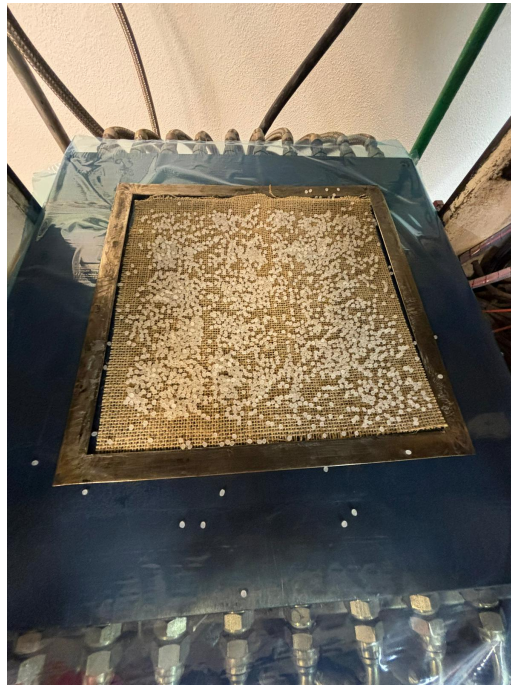
Figure 4.9: Layering Jute Fabric and PLA Pellets in the Mold.
