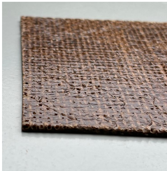
Figure 4.4: Jute Fibers Embedded in PLA Matrix.
