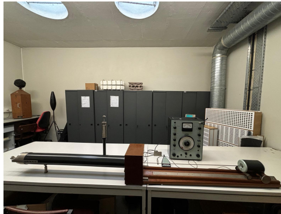
Figure 4.13: General Layout of the Impedance Tube Sound Absorption Test.
