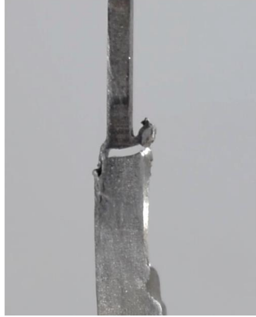
Figure C.3 - Localized yielding after main failure at the middle zone of the joints VII • (a) and VII •• (b).
