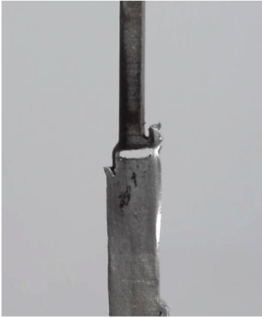
Figure C.3 - Localized yielding after main failure at the middle zone of the joints VII • (a) and VII •• (b).
