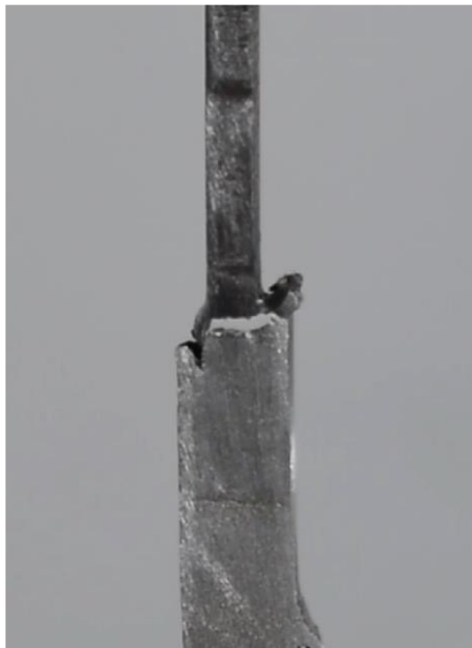
Figure C.4 - Localized yielding after main failure at the middle zone of the joints VIII • (a) and VIII •• (b).
