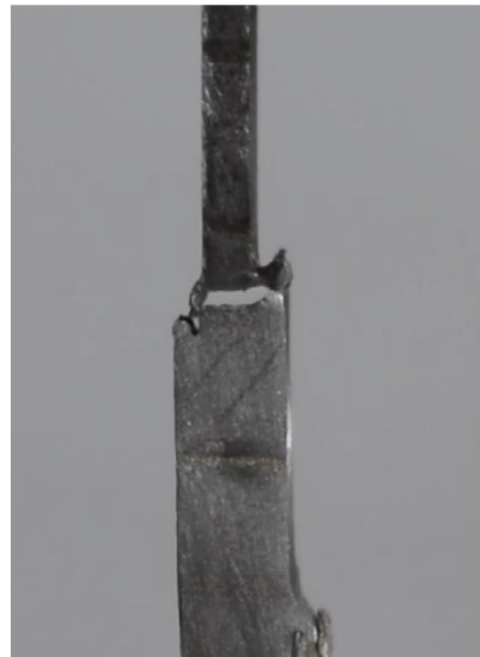
Figure C.4 - Localized yielding after main failure at the middle zone of the joints VIII • (a) and VIII •• (b).
