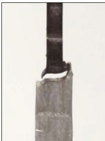
Figure 3.30 – Specimen II • • • tensile test video frame before the secondary failure instance, at the top zone of the joint.
