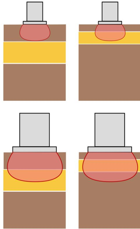
Figure 3. Different building widths and soil profiles
