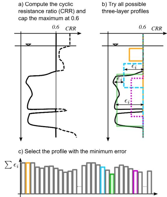
Figure 5. Procedure to implement the CRR-fitted method (after [20]).
