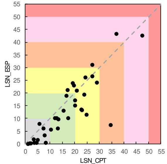
Figure 11. Comparison of LSN from CPTu and ESP
