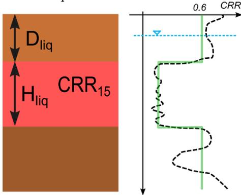
Figure 4. Definition of Equivalent Soil Profile (ESP)
