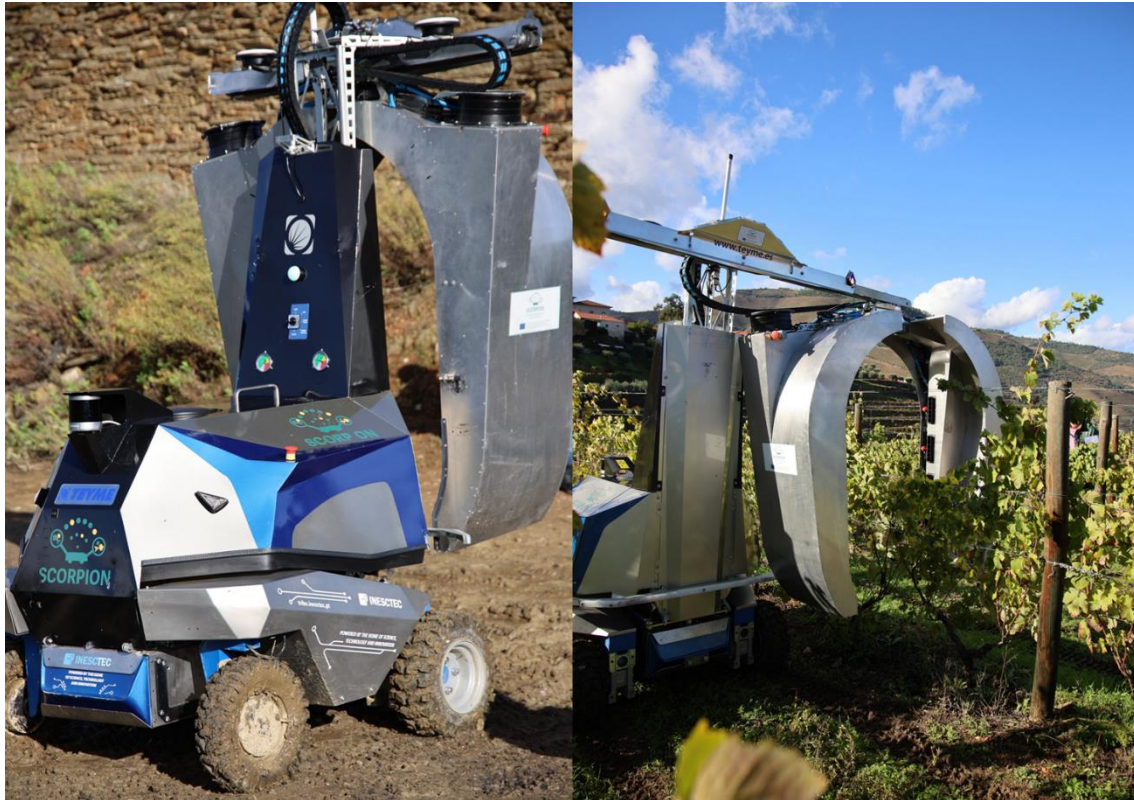
Figure 1 WETA Agro Robot: a hardworking autonomous platform conceived for helping people in agriculture and forestry developed under the scope of the SCORPION H2020 project (SCORPION 2022, INESCTEC 2024).
