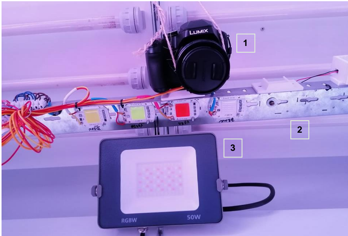
Figure 2 Set-up composed of an RGB camera (1) in combination with different light sources including individual Red, Green, Blue, and White LEDs (2) mounted on an aluminum plate, and a floodlight (UV and RGBW) (3).
