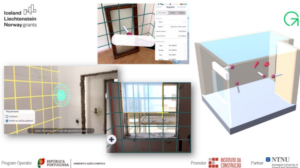
Fig. 5. LiDAR scan process in iPad as part of a diagnosis process.
