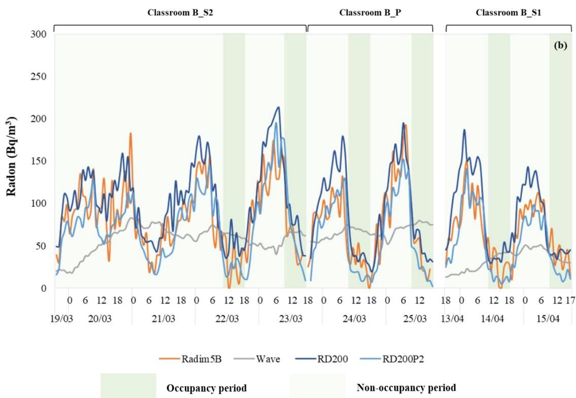
**Figure 1.** Time-series plots of radon concentrations in all studied classrooms from (a) Building A and (b) Building B.
