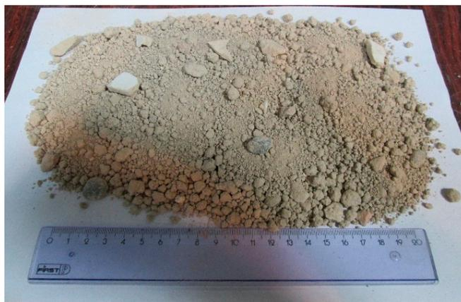
**Figure 2.** Visual appearance of the recycled C&D material used in this study.
