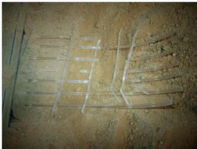
**Figure 8.** Detail of the transversal element rupture of the geogrid (at the end of pullout test).
