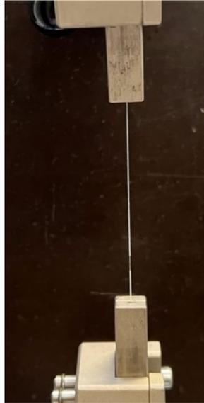
**Figure 3.9** Uniaxial tensile test to a filament of medical-grade PCL.
