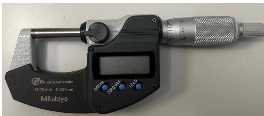
**Figure 3.7** The micrometre used to verify the filament thickness of the printed meshes.
