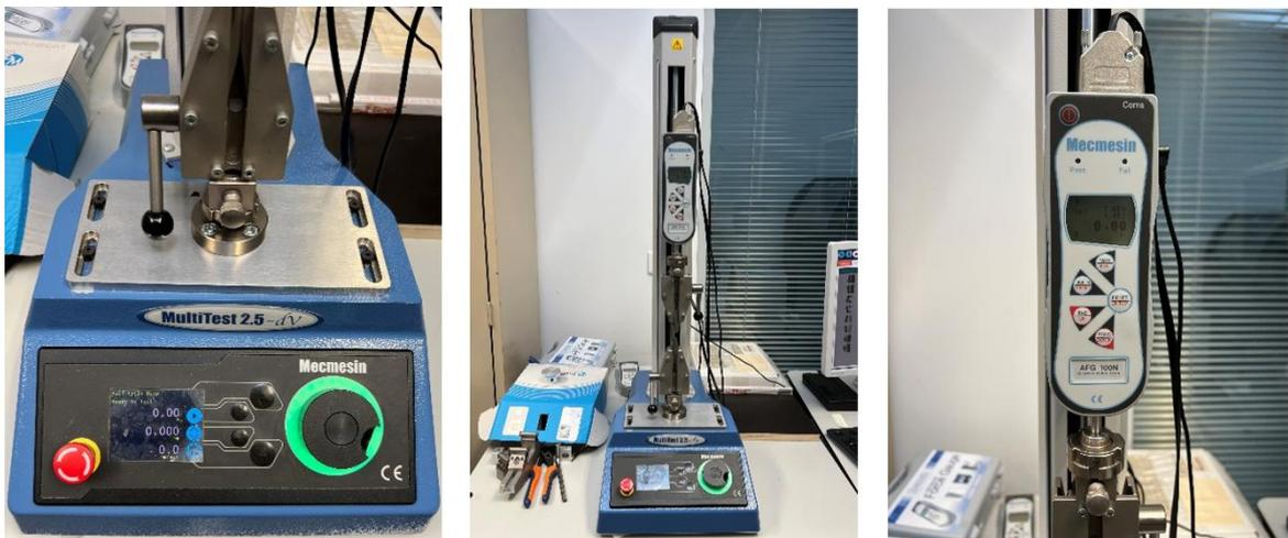
Figure 3.4 Uniaxial tensile test machine used to perform uniaxial tensile tests in samples of printed meshes.
