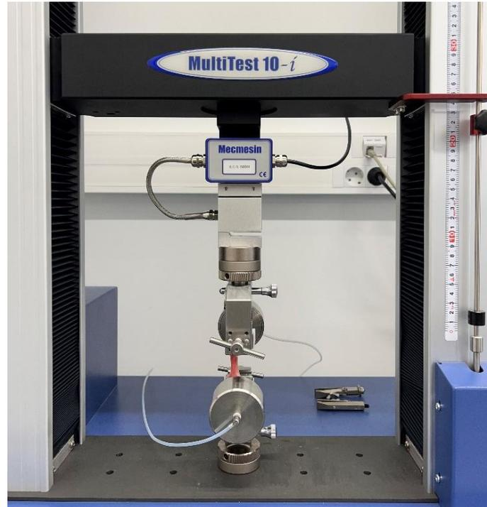
**Figure 3.5** Uniaxial tensile test machine used to perform uniaxial tensile tests in samples of vaginal tissue.
