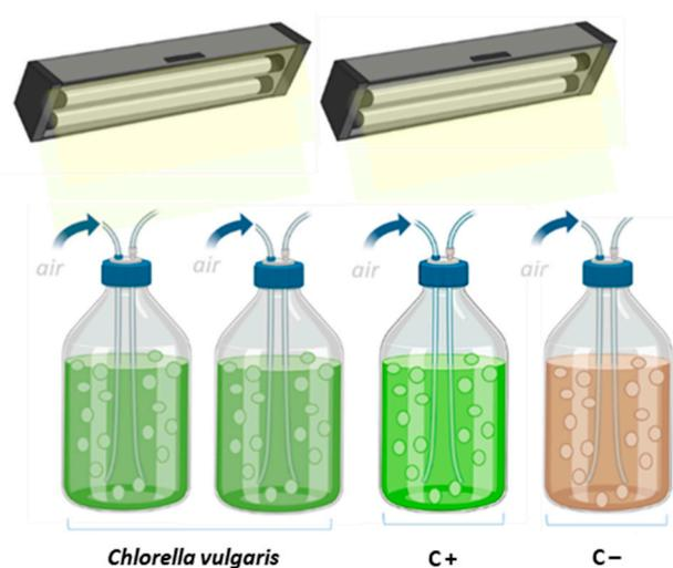
**Figure 1.** Experimental setup of the microalgal treatment, including the CV (*C. vulgaris* + UWW) PBR, positive (C+, *C. vulgaris* + autoclaved UWW), and negative (C-, UWW) PBRs controls.
