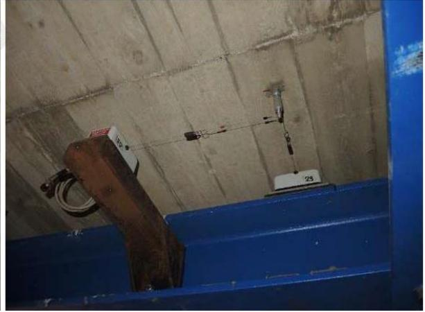
Fig. 3.10 – Wired Displacement Sensors at the 2<sup>nd</sup> Floor (ISAAC technical report, (2020))
