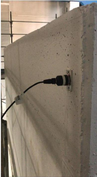
Fig. 3.11 – Piezoelectric accelerometer to measure the floors' acceleration (ISAAC technical report,
