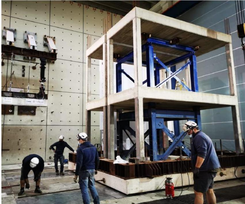
Fig. A.2 – Transport of the RC frame and the security steel structure to the shaking table (ISAAC technical report, 2020)
