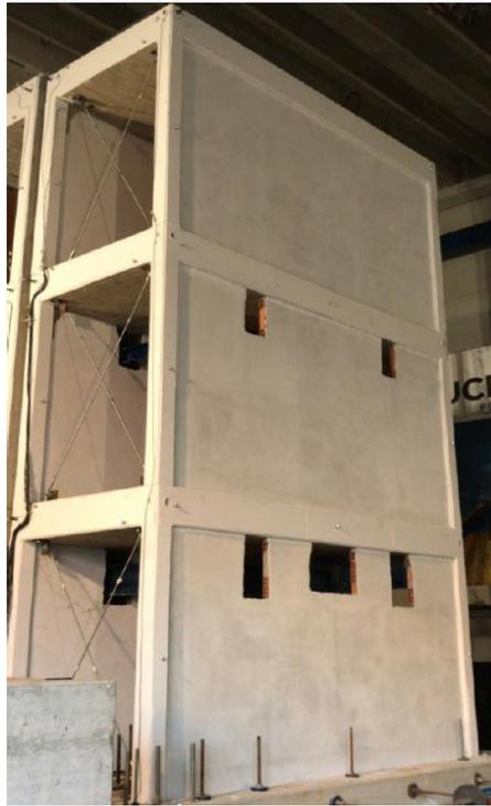
Fig. 3.2 – Specimen RC frame building (ISAAC technical report, (2020))
