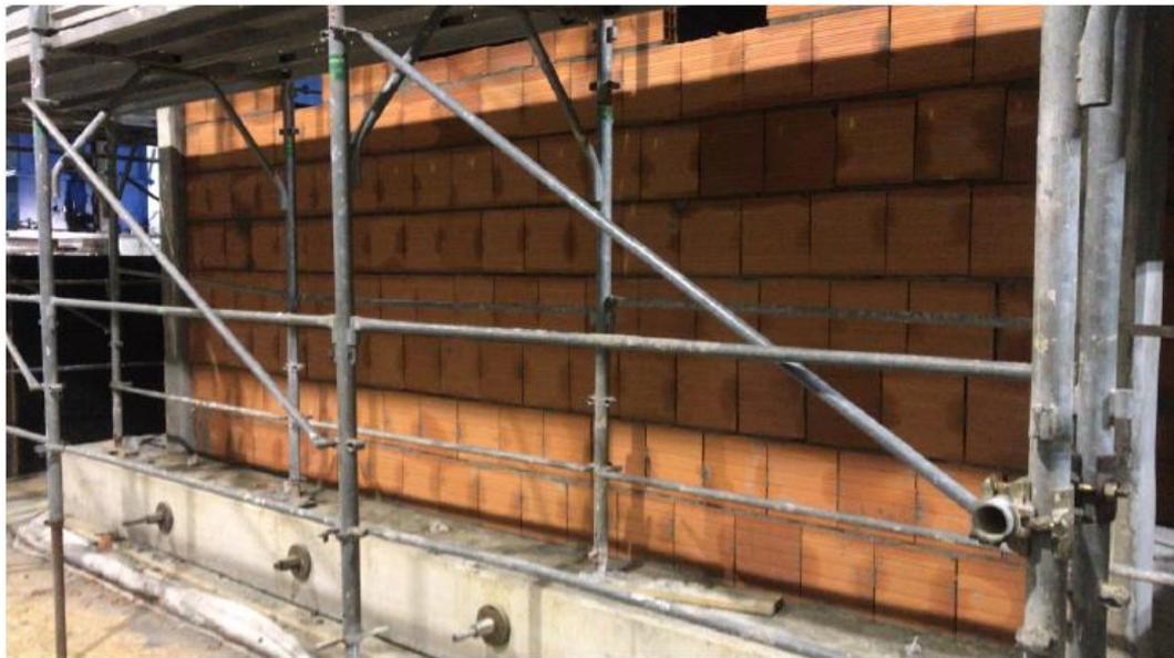
Fig. A.5 – Filling of the 1st storey bay with hollow clay brick units (ISAAC technical report, 2020)
