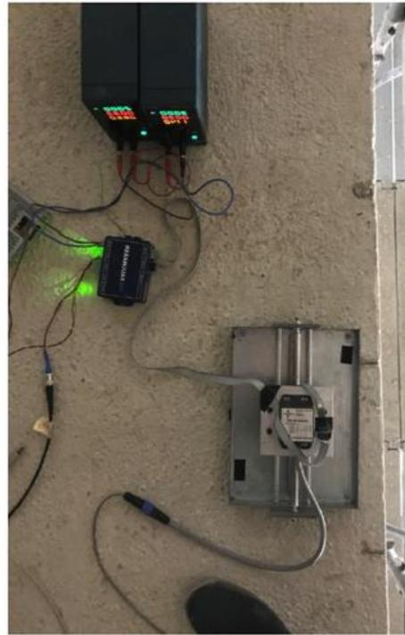
Fig. 3.12 – The 1.5 kg Vibrator at the highest floor (ISAAC technical report, (2020))
