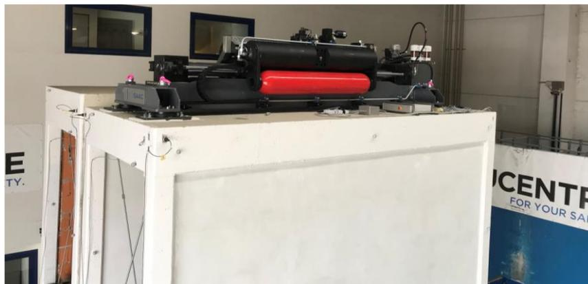
Fig. 3.1 – Active Seismic Damping System (ISAAC technical report, (2020))
