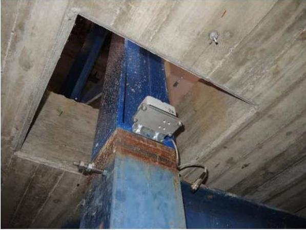
Fig. 3.9 – Wired Displacement Sensor at the 1<sup>st</sup> Floor (ISAAC technical report, (2020))
