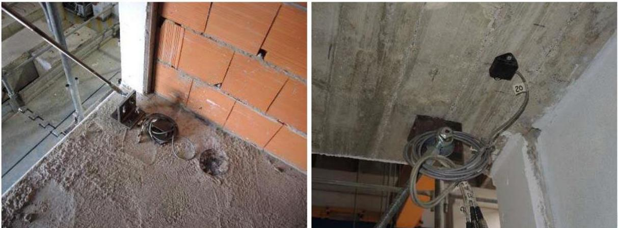
Fig. 3.8 – Accelerometers installed at the floors (Extrados and Intrados) (ISAAC technical report, (2020))
