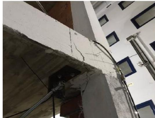
Fig. 3.23 – Observed cracks at the slab joints (ISAAC technical report, 2020)
