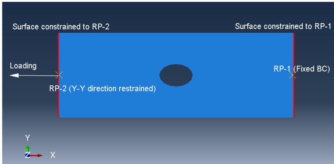
**Figure 4:** Loading and boundary conditions.
