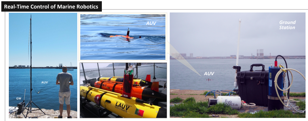
Figure 1.2: A set of illustrative examples of an AUV in real-world operation. It includes the so-called Manta gateway (GW) on the right and left pictures. The two middle image shows an AUV on the water (middle-top) and outside the water (middle-bottom) on a boat before a mission.
