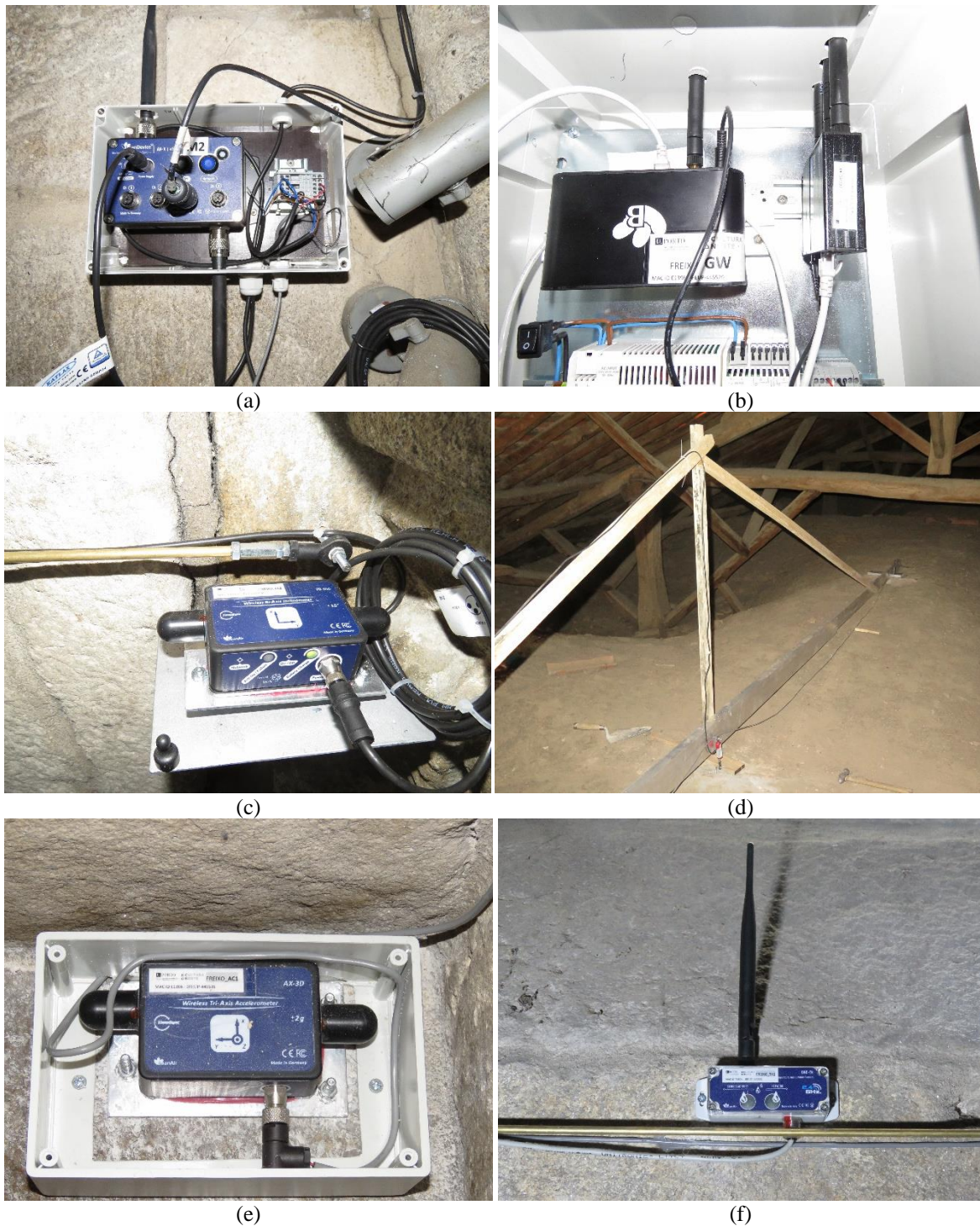
Figure 5. Monitoring system installed: (a) acquisition module M2; (b) gateway; (c) tiltmeter (CL2) and extremity of crackmeter FS3; (d) crackmeter FS7 installed on the extrados of the vault; (e) accelerometer (AC1); (f) temperature sensor TH1 and the extension rod of the crackmeter FS2 [source: authors].
