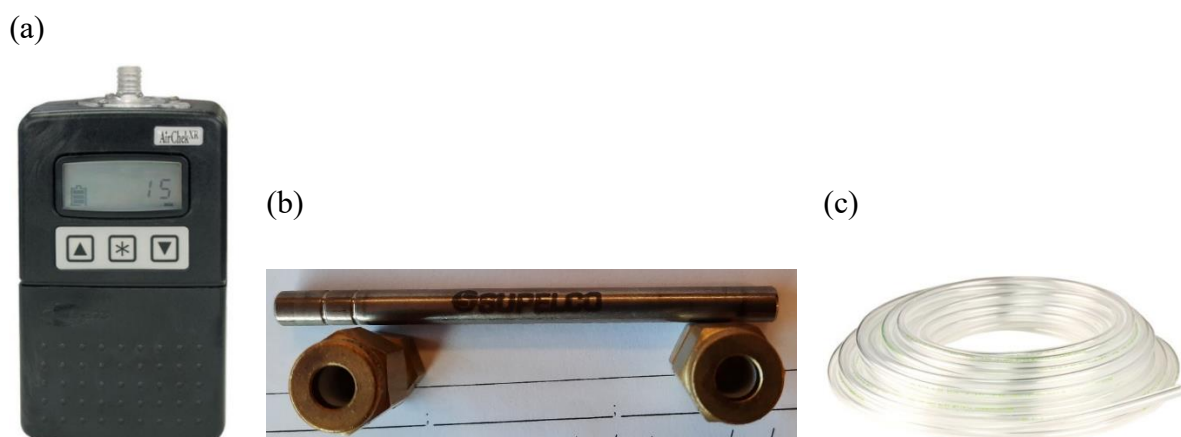
Figure 3-2 - Representation of sampling system: (a) AirChek XR5000 (SKC Ltd) pump; (b) Stainless-steel sorbent tube (Tenax TA; 60/80 mesh); (c) Tygon® high-purity tubing
