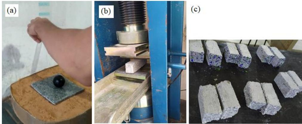
**Figure 2.** Tests procedures. (a) Hard body impact strength, (b) Tensile strength, and (c) Halves of specimens.
