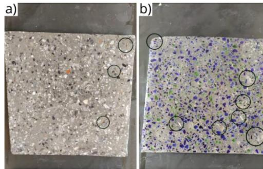
**Figure 3.** (a) Specimen with natural aggregate, and (b) Specimens with glass waste aggregate.
