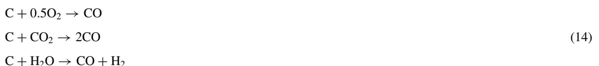
Regarding the kinetic rate of reactions in the present model, data was obtained from [24,25]. Many factors influence the heterogeneous reactions, such as reactant diffusion, breaking up of char, and interaction with the
