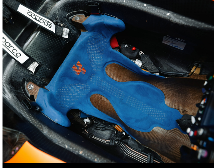
Figure 1.6: McLaren's Formula 1 car seat made of flax fibers [Bcomp, 2022]
