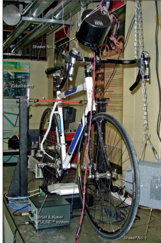
Figure 2.13: Setup for SIMO and MIMO analysis [Champoux et al., 2007]
