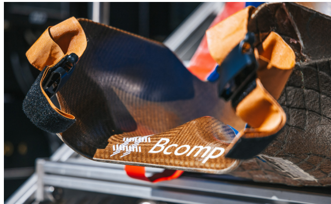
Figure 1.7: McLaren's Formula 1 car seat made of flax fibers [Bcomp, 2022]
