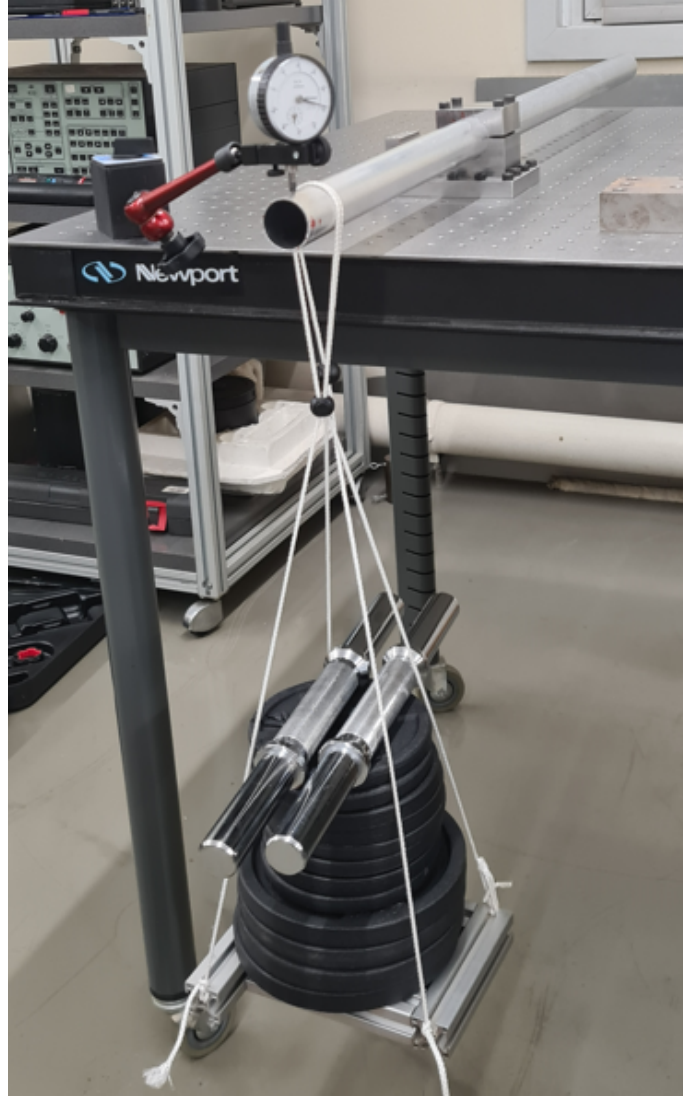
Figure 3.1: Setup for the stiffness test of the cylindrical tube
