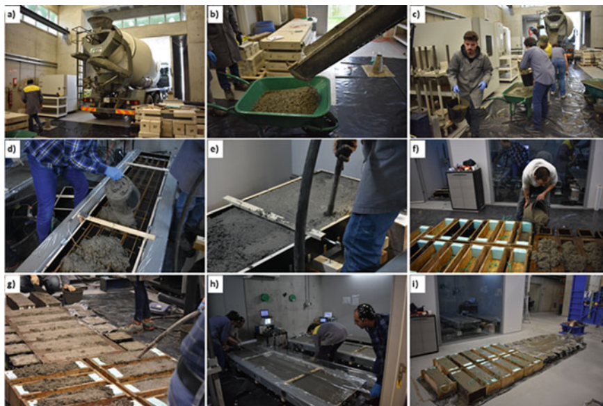
Fig. 7 Casting of the long-term experimental campaign: a arrival of concrete truck; b filling the wheelbarrows; c transportation of concrete buckets; d casing the slab specimens; e vibrating slab specimens; f casting load blocks and characterization specimens; g vibrating load blocks and characterization specimens; h sealing the test specimens; i sealing the characterization specimens
