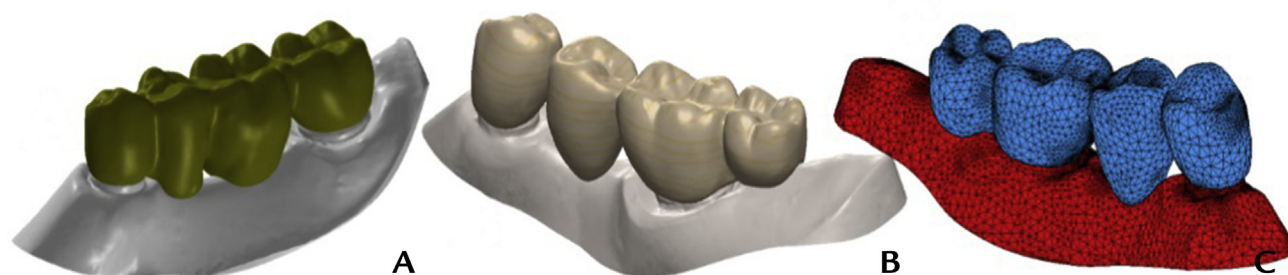
Figure 3. A, B, Digital models of test prostheses reconstructed by using computer-aided design software program. A, Conventional. B, Cantilever. C, Finite element model developed by using nonlinear software package.
