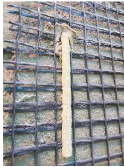
Figure 4: Specimen R2-OOP: Detail of the L-shape connector.
