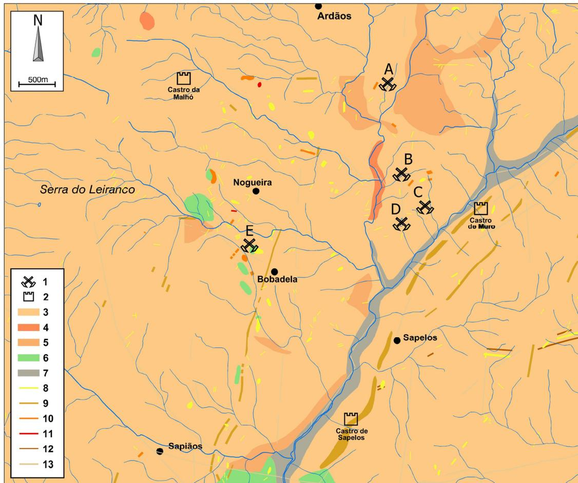
Fig. 1. Geological map of study area modified from Chaves 6-B Portuguese Geological Map 1:50.000 scale (1967): 1 – Ancient Gold Mine; 2 – Hillfort; 3 – Regional granite; 4 – Coarse granite; 5 – Fine granite; 6 – metasediments; 7 – alluvial sediments; 8 – Quartz veins; 9 – Quartz thick barren veins; 10 – Mineralized quartz veins; 11 – Pegmatite vein; 12 – Basic rock vein; 13 – Faults. A) Batocas; B) Limarinho; C) Ribeira do Calvão; D) Poço das Freitas; E) Lagoa do Brejo.
