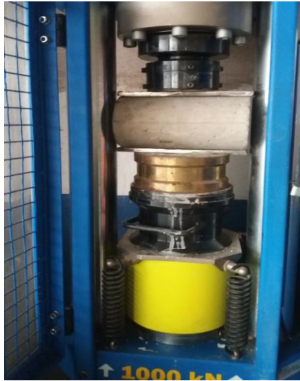
Figure 6. Tensile strength test.
