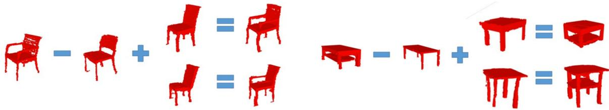
Figure 3.21: Arithmetic operations of the 3D-GAN. The left example shows how to add arms to a chair and the left example how to add layers to a table [45].
