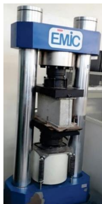
Figure 7. Testing the block compressive strength on the Machine Model EMIC series 23.
