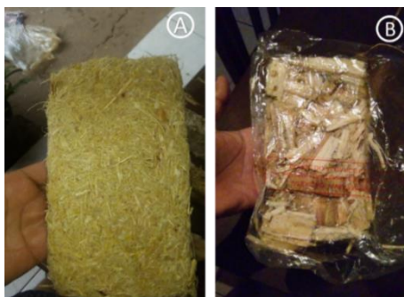
Fig. 9. Specimen: (A) fibers 2 mm granulometry and (B) protected with plastic bag.
