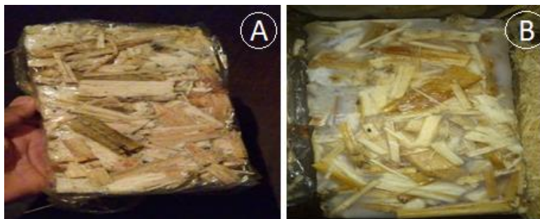
Fig. 8. Specimen with a particle size of approximately 1cm: (A) with white glue and (B) with resin.
