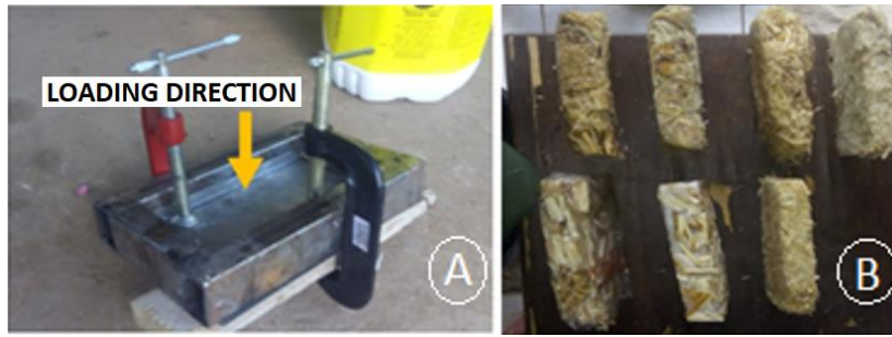
Fig. 5. Manufacture: (A) Prefabricated tools and (B) panels arranged vertically for curing
