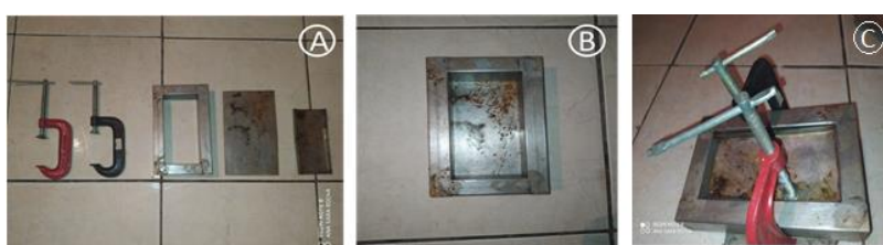
Fig. 3. Manufacture of the press: (A) tools and materials used, (B) the tray of the press and (C) press mounted to mold the panels.
