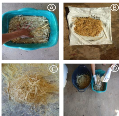
Fig. 1. Processes performed: A) submerged bagasse, B) drying of bagasse in sunlight, C) crushed bagasse and D) mixing of resin with bagasse.
