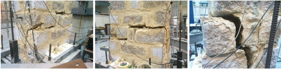
**Fig. 22** Horizontal crack with relative interleaf displacement (from OP PF2)
