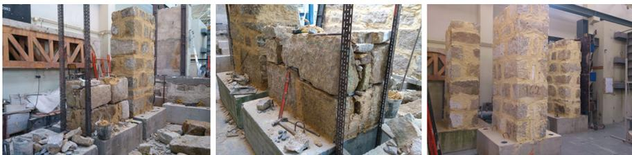
**Fig. 2** Construction and preparation of the masonry walls
