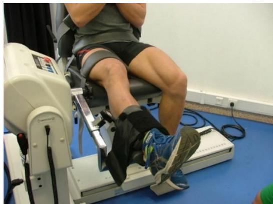
Figure 5 – Isokinetic Dynamometer positioned at 60 degrees.
