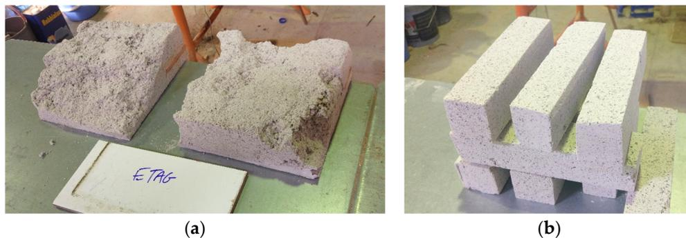
**Figure 4.** (a) Original pieces of the mortar with the protective coating on their surface after wall removal; (b) prismatic specimens after cutting from original pieces.
