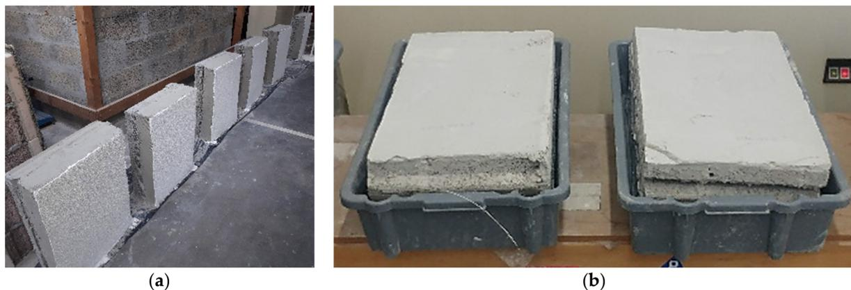
**Figure 2.** (a) Small-scale specimens ( $0.6 \times 0.4 \text{ m}^2$ ); (b) humidification/thawing procedure.
