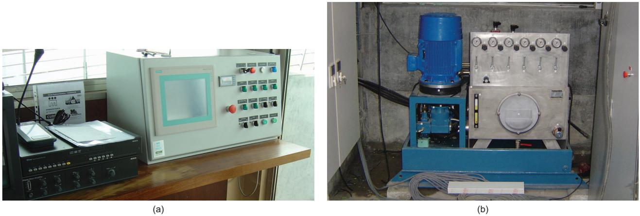
**Figure 15.** Touch-screen control panel (a) and hydraulic power pack (b)
