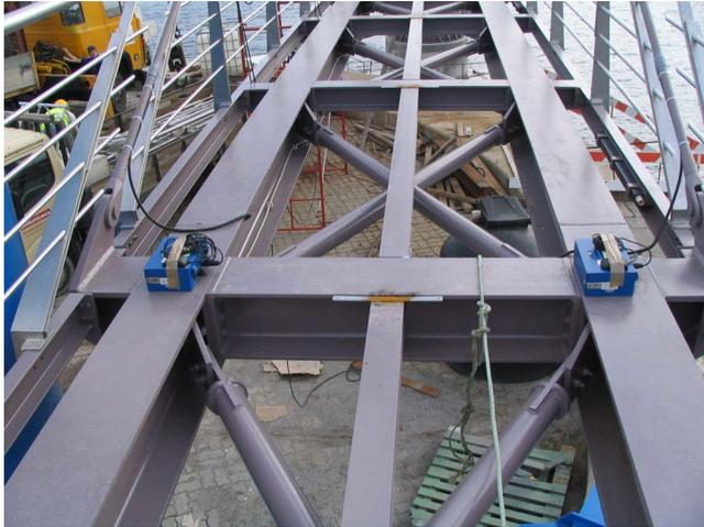
**Figure 18.** Bridge deck during the first ambient vibration test and two measuring units
