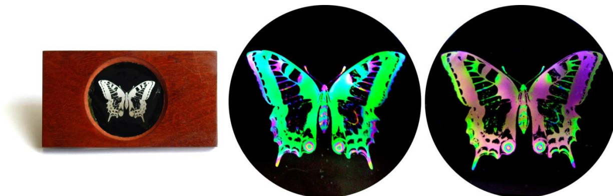
Figure 14. Gypsum preparation for projection in polarized light. Complementary colours as shown by the 90° rotation of the nicol.
