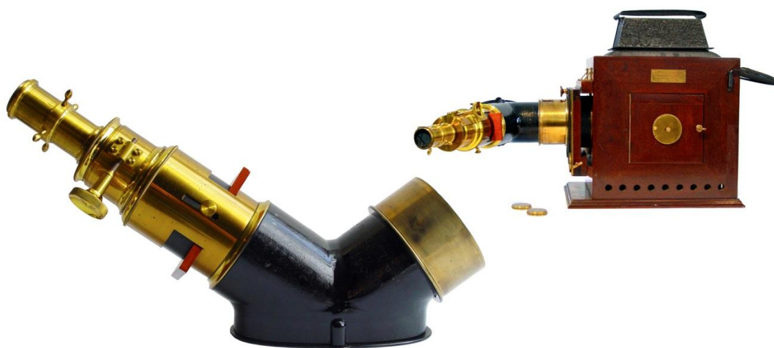
Figure 13. Elbow polariscope attachment and fitting procedure.
