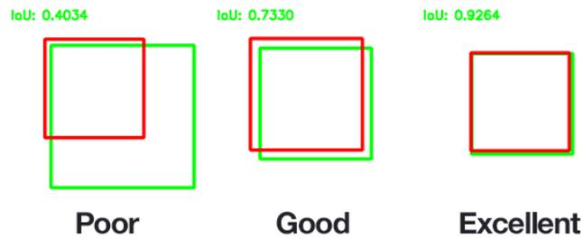
Figure 2.9: Example of IoU values for different bounding boxes [6].
