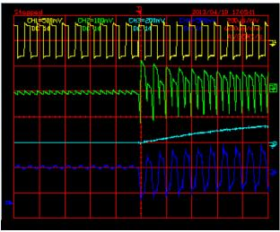
Fig. 4. Dynamic test with variable duty ratio. Vh (Ch1- yellow: 100V/div), Ic (Ch2- green: 5A/div), Ibat (Ch3- cyan: 2A/div), IL (Ch4- blue: 5A/div).
