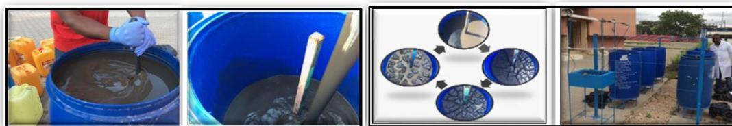
**Figure 2:** Homogenization and filling of the drying beds; start-up of the operation and monitoring of the system; evolution of sludge drying inside the beds.
