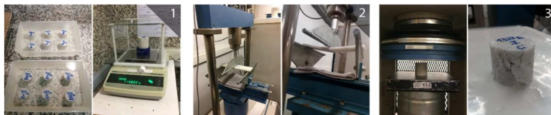
Figure 5. Tests carried out; (1) apparent density and water absorption, (2) flexural strength (bending) and (3) compressive strength.
