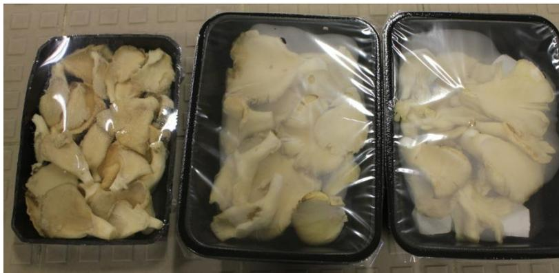
Fig. 8.1 – Examples of the packages used in the experiment. Commercial package; modified atmosphere package and modified atmosphere package with moisture absorber, respectively.
