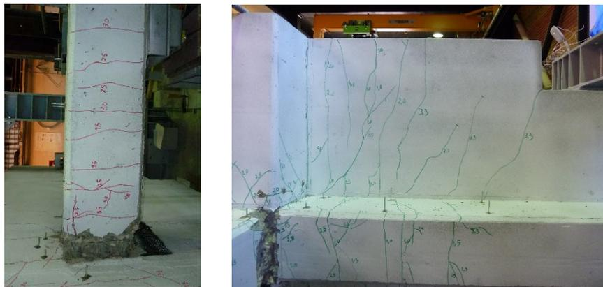
Fig. 8. Final damage state in C-EC8; left: superior column, right: beam underside
