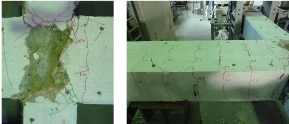
Fig. 4. Final damage state in C-noSLT; left: joint, right: beam
