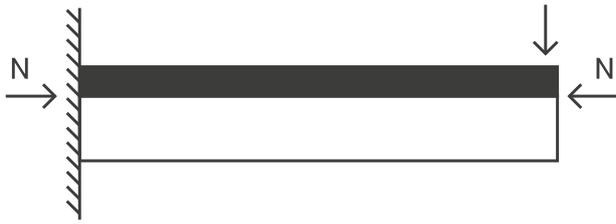
The cables introduce compressive stresses that reduce the deformation under vertical loads.
