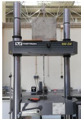
Figure 1. The pull-out test set-up.
