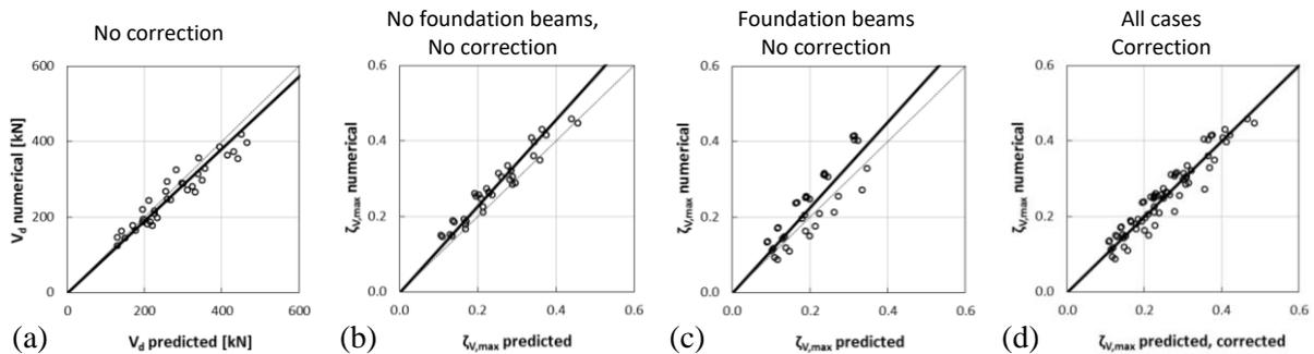
Figure 5. Predicted vs. numerical results of  $V_d$  and  $\zeta_{V,\max}$
