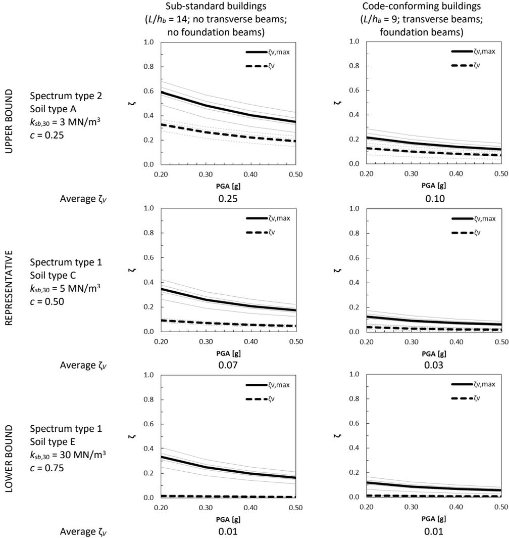
Figure 9. Values of relative shear force ( $\zeta_v$ ) due to settlement depending on the PGA of the seismic event for different situations;  $h = 3$  m,  $h_b/b_w = 1.5$ ,  $w = 6.6$  kN/m<sup>2</sup>,  $q = 100$  kN/m<sup>2</sup>; thick line denotes average values
