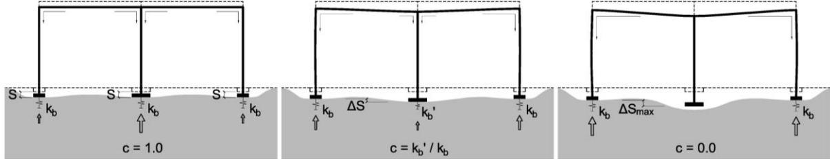
Figure 1. Conceptual configurations of equivalent models and  $\Delta S$  for decreasing values of  $c$
