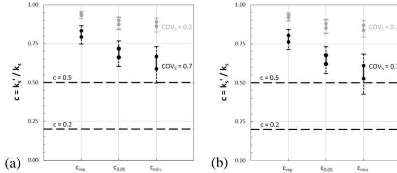
Figure 7. Representative ( $c_{rep}$ ), characteristic ( $c_{0.05}$ ) and minimum ( $c_{min}$ ) equivalent soil degradation parameter according to different geometric and probabilistic assumptions, for  $\Delta H = 4B$  (a) or  $6B$  (b)
